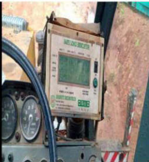
Fig-16: Automatic Safe Load Indicates Installed at all Lifting Crane
